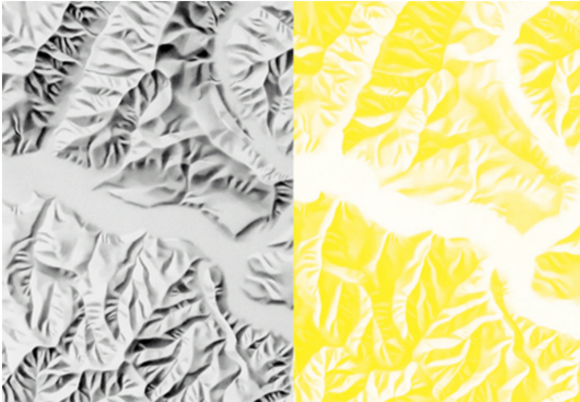
Figure 4. Left: Grayscale shading from a map of the Federal Office of Topography swisstopo at 1:25,000. Right: The reverse of the same shading in yellow. Flat areas have been masked.
