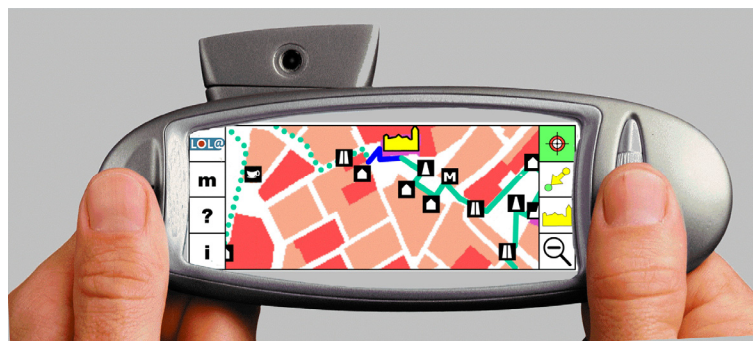
Fig.5: Display with integrated soft-keys
