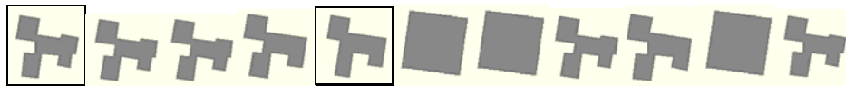
Figure 4 : Building generalisation by a micro-agent (5 constraints: Size constraint, Granularity constraint, Squareness constraint, Width constraint, Concavity constraint)
