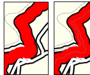
Figure 3 - Road Junction conflict: the left white road seems to end in the bottom curve of the biggest road while it is actually connected to the top curve.
