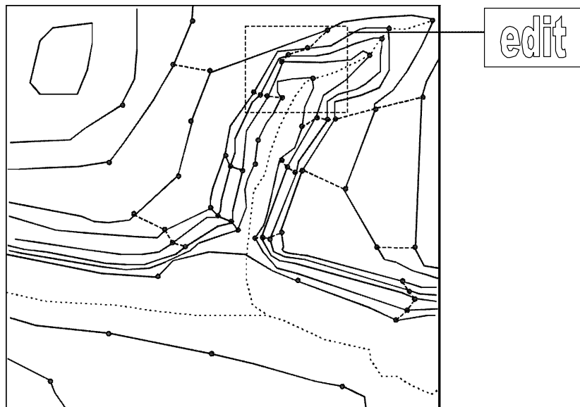
Fig.13 (c) The result of the intersecting data handling, after manual editing Fig.13 The process of progressive contours generalization
