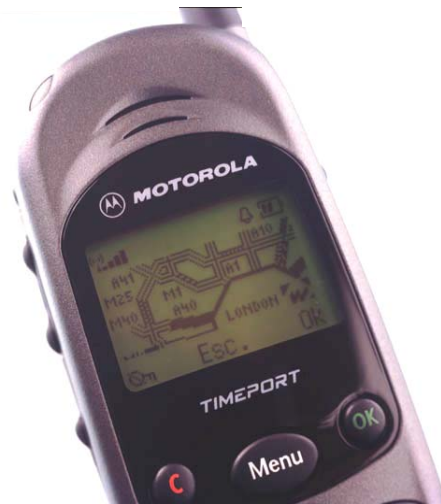
Figure 1: An example of a WAP enabled Internet phone displaying a map (Motorola L-Series)
