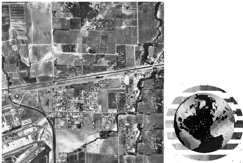
Figure 3. Watermarked Digital Aerial Photo (left) and Recovered Signature Image after 74% JPEG lossy compression
